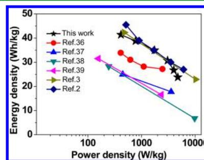
Figure 5. Ragone plots of the asymmetric supercapacitors and performances of references.
