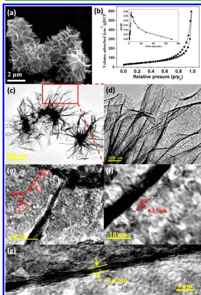
**Figure 1.** Ultrathin and porous features of Ni–Co sulfide nanosheets (Ni–Co–S-6). (a) SEM image of the prepared Ni–Co sulfides. (b) Nitrogen adsorption–desorption isotherms of the ultrathin Ni–Co sulfide nanosheets and (inset) Barrett–Joyner–Halenda (BJH) pore size distribution. (c–f) TEM and HRTEM images of the Ni–Co sulfides. (g) Vertical HRTEM image of Ni–Co sulfide nanosheets.
